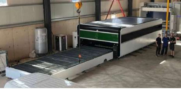
GWEIKE LASER 2500x6000 - 12kW laser power
